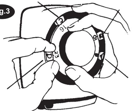
3. Ensure that the installer has removed the protective tape covering the pre-selector wheel.
